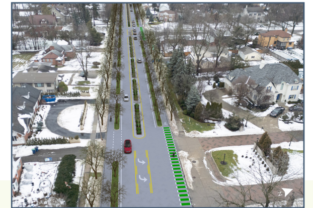
Renderings of the 3 Lane Option (with enhanced pedestrian and bike facilities on both sides); see pages 28-29 for more information.
